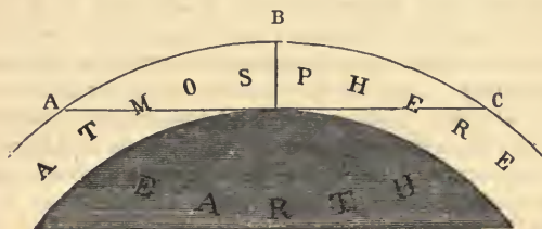
FIG. 8.—Diagram showing the influence of the varying thickness of the atmosphere in retarding the Sun's heat. A. Line of the Sun's rays at sunrise. B. Line of the rays at noon. C. Line of the rays at sunset.
